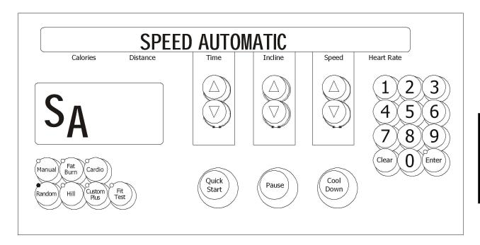
Upon entry into this test the letters SA (speed automatic) will be in the profile window. This test allows the user to test the main drive motor and controller controlling the target speed. The user can select a target speed by using the speed arrow keys. The actual speed as calculated by the speed feedback sensor is shown in the actual portion of the message center.
